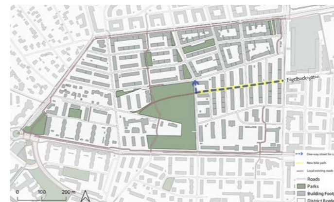
Fig 37. This map is showing new bike path and one-way street for cars.
